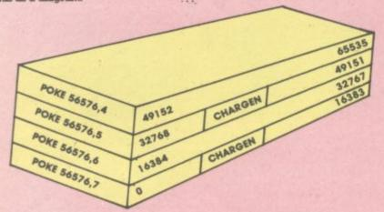
We can control which slice we want by manipulating the two low bits in address 56576 (hex DD00). Normally, the processor picks the slice from 0 to 16383.
